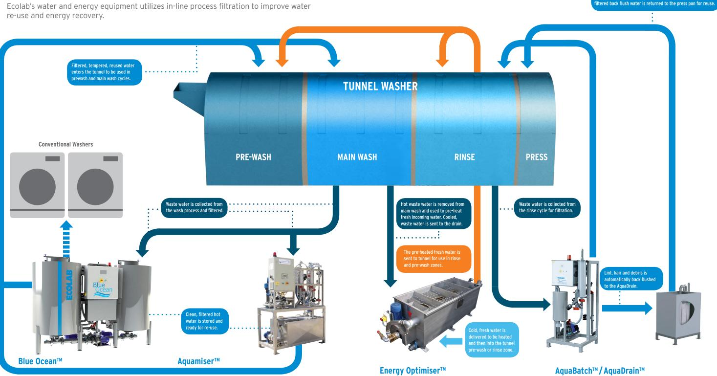
The most efficient and reliable system has the capacity to recover up to 4,000 gallons per hour. Waste water is removed from the wash process and filtered. The cleaned, already heated water, is then sent back to either tunnel or conventional machines for a new wash cycle.
