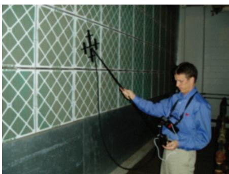
Figure 7 - Illustrates the part of the data collection method used to calculate energy use before and after a cleaning
