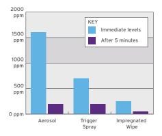
\*TECHNICAL REPORT - TR9902R Investigation into Airborne Concentrations of Alcohol when using a Trigger Spray, and Aerosol and Impregnated Wipes
