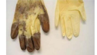
Figure 7: Nitrile gloves after one week's exposure to lotions at 50°C
