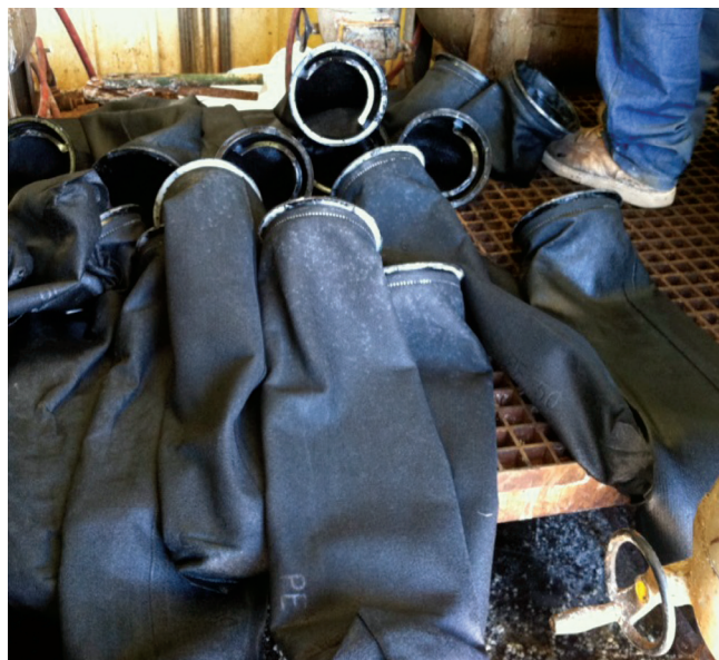
Figure 1 - Fouled sock filters prior to injection of BIOC16734A.
